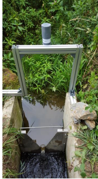
Ultrasound sensors (inlet & outlet)
