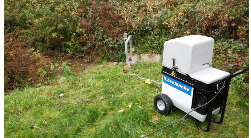
Automatic and chilled samplers (inlet & outlet) controlled by the flow rate
