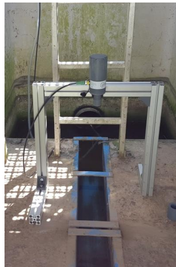
Ultrasound sensors (inlet & outlet)
